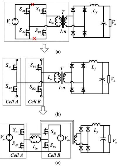
**Figure 1.** Proposed full bridge 3 port converter. (a) Full bridge converter. (b) 2 switching cells. (c) Full bridge 3 port converter
