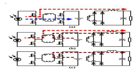
Figure 3. Power flow directions of each operation mode, (a) DO mode. (b) DI mode. (c) SISO mode.
